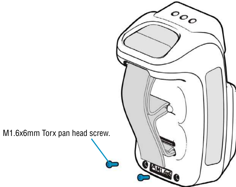
FIGURE 10: Battery cover locking screw location
