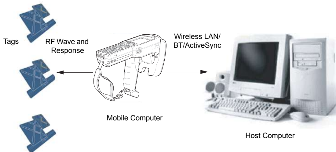
Figure 1-1 RFID System Elements
