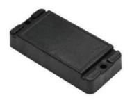
Rhino HT-HTP 6229 is a High Temperature RAIN (UHF) RFID tag optimized for metal substrates that has the ability to survive temperature of 260°C for extended periods. With a rugged encapsulation, this RAIN (UHF) RFID tag is ready for deployment in a variety of applications without compromising read range performance.
